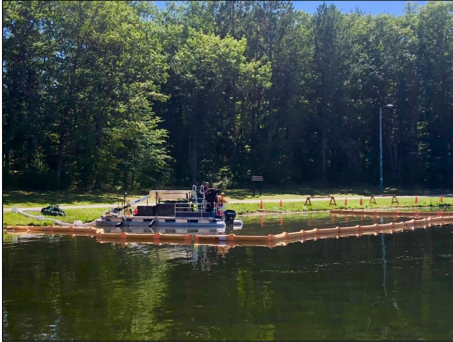
Figure 57. A DASH boat used in a lake for aquatic plant removal.
