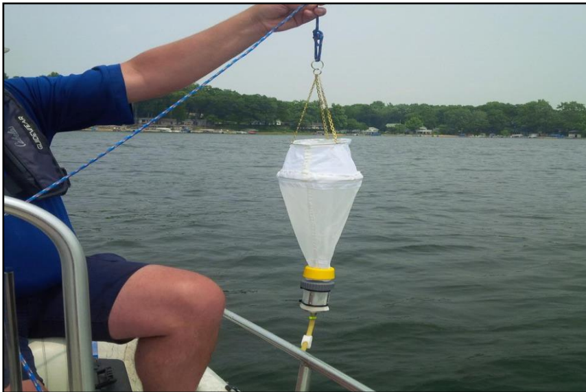
Figure 31. A zooplankton collection tow net.
